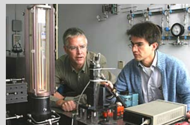
Chris Shaddix, left, and Alejandro Molina discuss an experiment to determine the best proportion of oxygen and CO 2 for oxy-combustion of coal.
